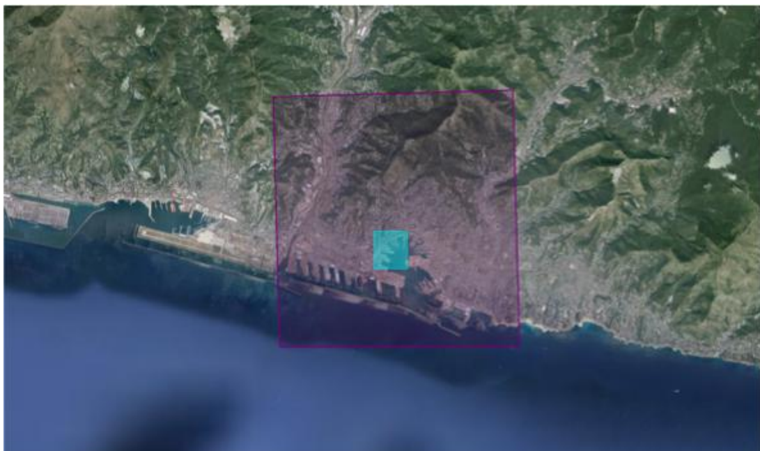
Fig. 2.2.2.2 – Simulation domain for the Genoa area. The cyan box includes the touristic harbor and the violet box show the simulation domain.
