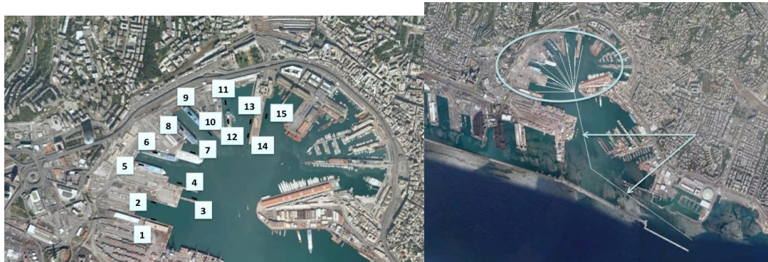
Fig. 2.2.2.1 – Passenger ships emission sources in Genoa area simulations. On the left ships in hoteling phase, on the right ships in maneuvering phase.
