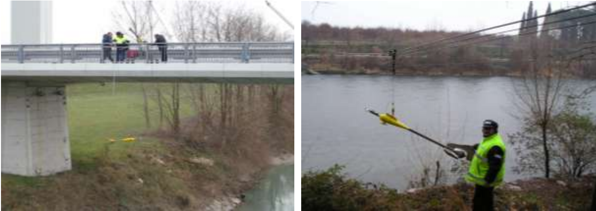
Figure 8: Different techniques for flow velocity measurements; from bridge and using a cable
