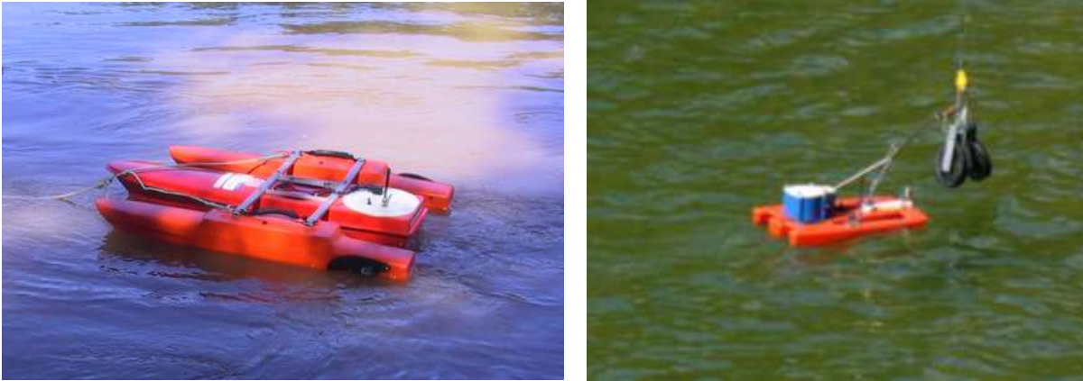
Figure 10: ADCP RioGrande (for moderate/high flow depths) and StreamPro (for low/moderate flow depths) models
