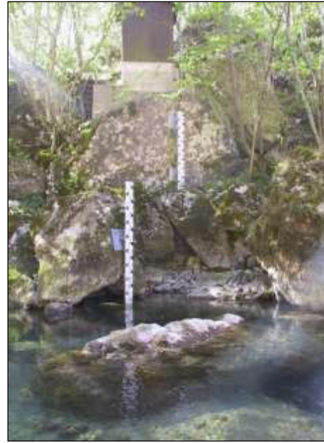
Figure 14: Hydrometric references; echo sounding automatic system and hydrometric rod for water level gauge
