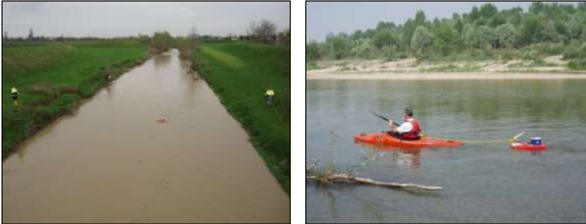
Figure 12: ADCP measurements from bank to bank and by canoe
