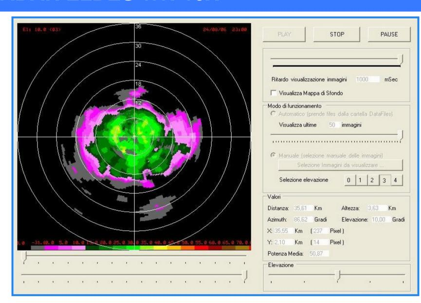
The GUI allows the visualization of the data and the total control of the microradar. Remote control system is also available with the possibility of turning the instrument on/off, monitoring remote parameters (T, power supply,...).
