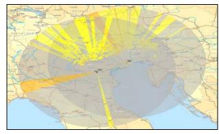
**Figure 1**. Example of scans being used for a particular scanning strategy over Veneto. The grey/yellow/orange colors represent data to be used from the  $1^{st}/2^{nd}/3^{rd}$  tilts respectively. The Teolo radar (LIZT) is to the southwest, Loncon (LIZL) is to the northeast.
