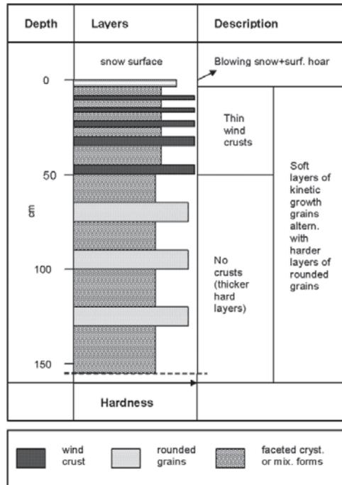
Fig. 1 - Schematic snowpack structure at Dome C (surface layers).
