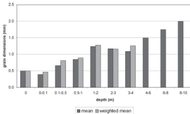
Fig. 3 - Average dimensions of grains for depth classes.
